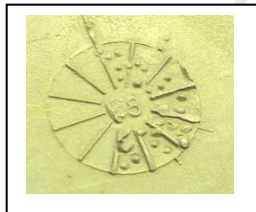
1969 alternator #28757749. The assy date is 34 th week of 1968 (Aug 17-21). casting date= 7 th month of 1968. Difference of 30 days (casting to assy)
