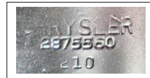
1970 starter part # 2875560 and assy date of 21 st week of 1970. The casting date on the solenoid housing was the 3 rd week of 1970.
